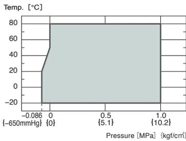
● Use after confirmation that the maximum operation pressure and maximum service temperature are within the operation range.
